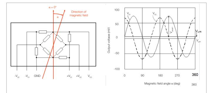
Fig. 1: *left*: Simplified circuit diagram with schematic of applied magnetic field.  $\it right$ : Output signals as a function of the magnetic field angle  $\alpha$ .
